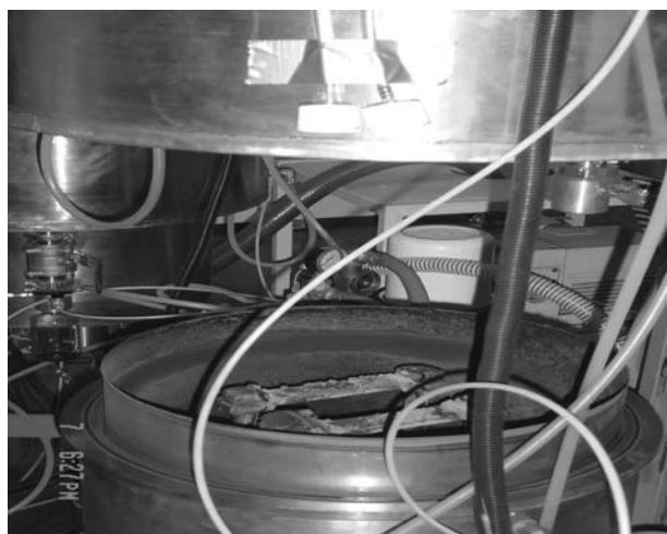
**FIGURE 2.** Reactor cleanout process with no fume extractor (LEV)
