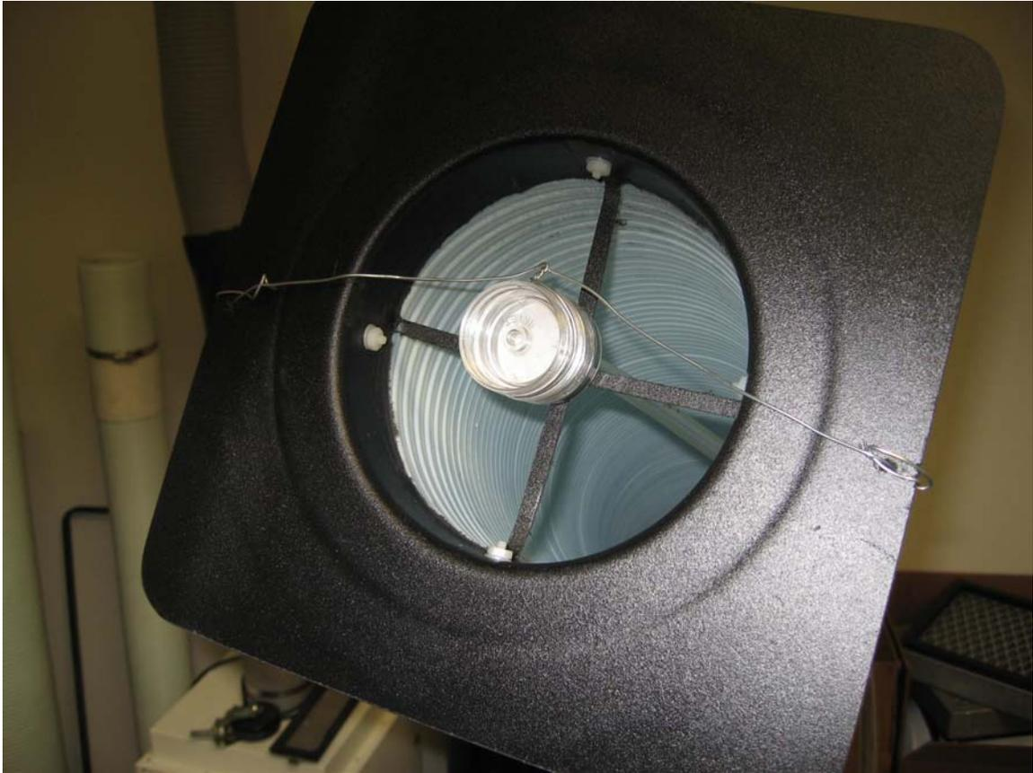
**Photograph #3: The inlet duct of the welding fume extractor is shown above. The sampling filter cassette was wired in place to permit sampling of the air being drawn into the extractor.**
