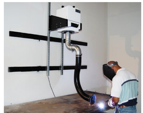
Model 300 Sky Sentry mounts on wall to free up needed benchtop space.
